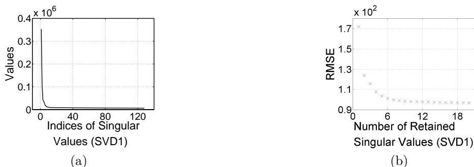
Figure 2. The singular values of the first singular value decomposition (Approximation Step 1) and their importance in the approximation. a. The singular values of the first singular value decomposition; b. The root-mean-square errors (RMSE) between the smoothed point spread functions and the experimental point spread function P_{exp} . The smoothed estimates are obtained by using different numbers of retained singular values in the first singular value decomposition (Approximation Step 1) but keeping 20 singular values of the second singular value decomposition and all singular values in the other singular value decompositions.
