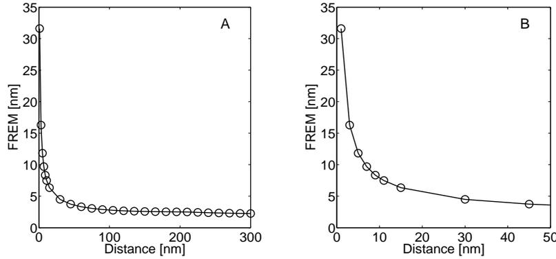
**Figure 1.** Panel A shows the FREM as a function of the distance of separation for a pair of TRITC molecules. Panel B shows the same for a distance range of 1 – 50 nm. In all the plots, the numerical aperture is set to be  $n_a = 1.45$ , the wavelength of the detected photons from the TRITC molecule is set to be  $\lambda = 600$  nm, the photon detection rate  $\Lambda_0$  of each TRITC molecule is set to be  $\Lambda_0 = 2500$  photons/s and the acquisition time is set to be 1 s.
